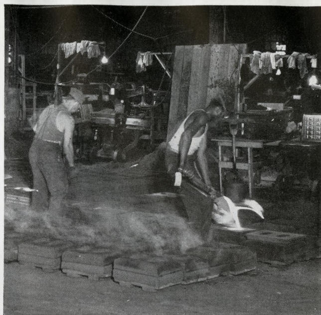
No. 3—Floor pouring—The tractors bring the iron to the molders who pour their own molds in this section of the foundry.
