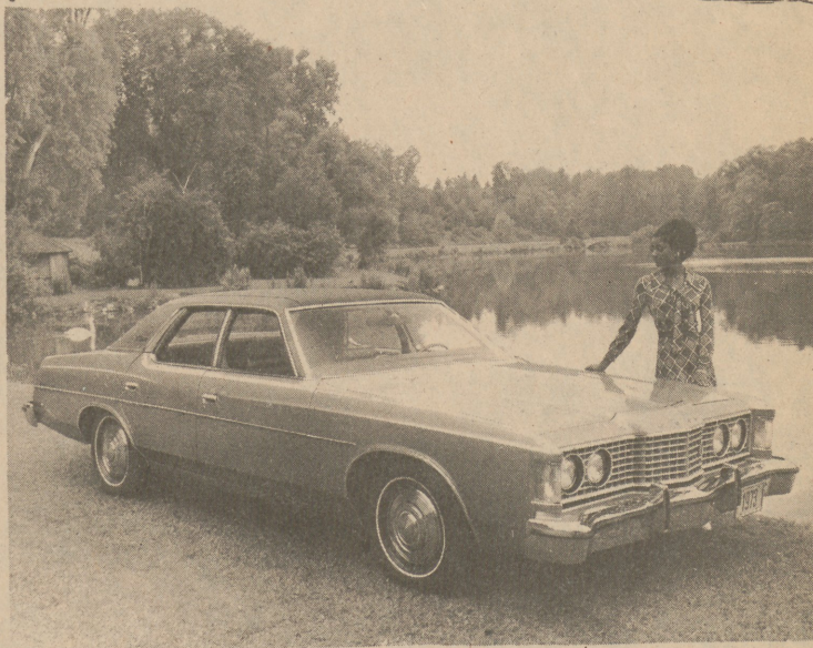
The 1973 Ford Galaxie 500, shown here in the four-door pillared hardtop model, is distinguished by a new front appearance and new sheet metal below the window line. For 1973 it features an improved rear suspension. A new window weather-stripping further improves the Ford quiet ride. Power is provided by a standard 351-2V eight cylinder engine and SelectShift Cruise-O-Matic transmission.
