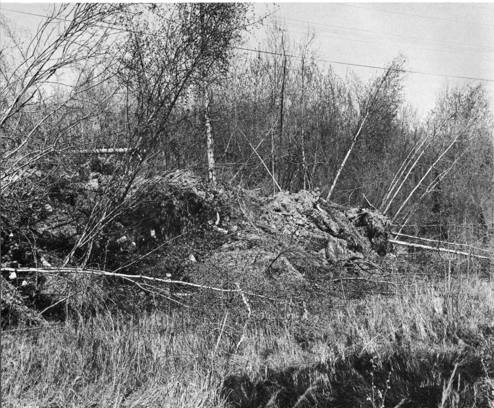
21.—Chaotic pressure ridge at toe of rotational slide, Bluff Road.. In part, toe surged forward as an earthflow. Compare with figure 22.
