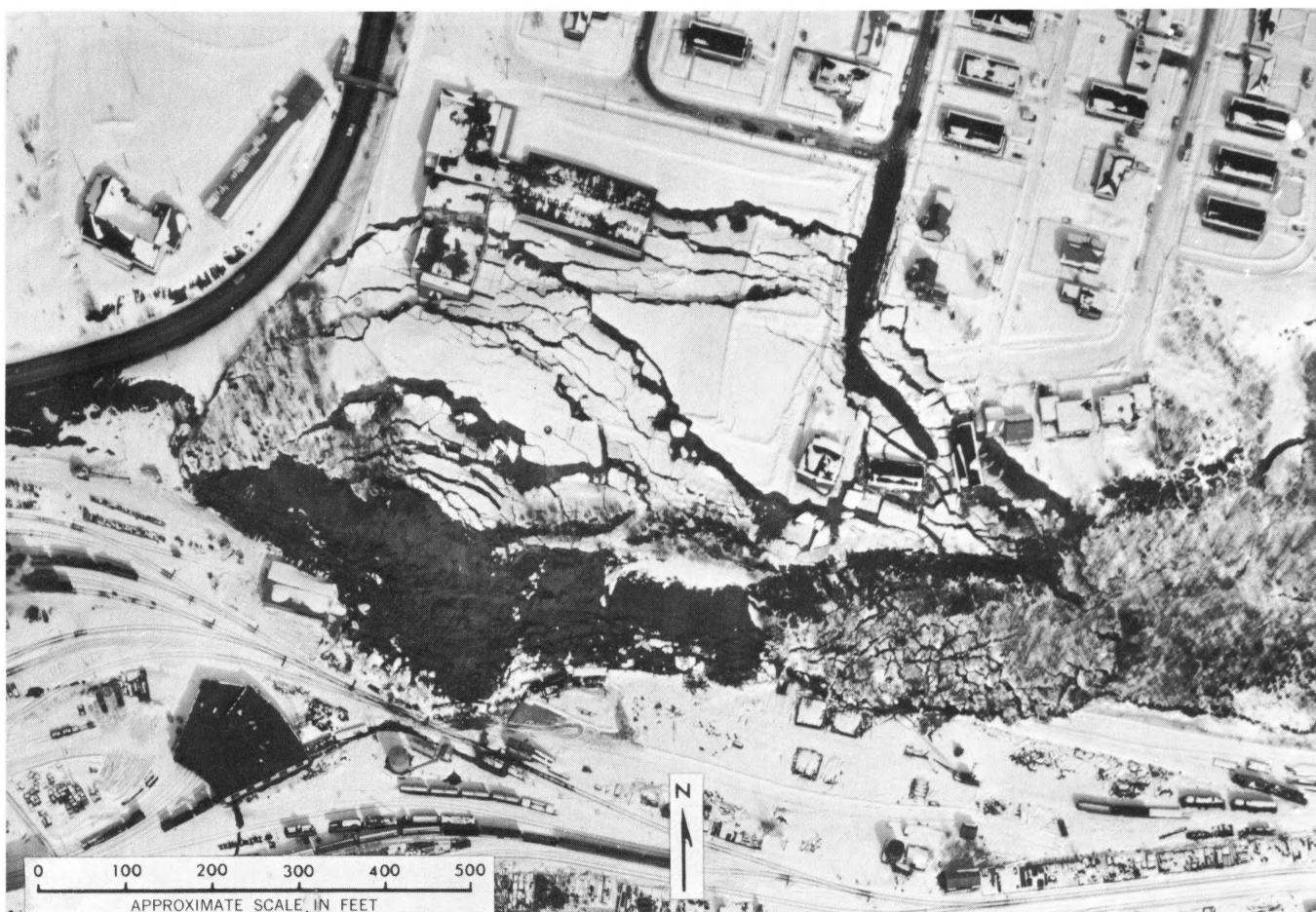
35.—Air view of Government Hill slide, Anchorage, Alaska. Graben plainly discernible. Compare with figure 38. Photograph by Air Photo Tech, Anchorage, Alaska.
