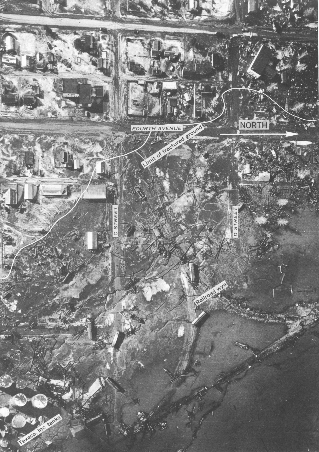
4. Aerial view of the northern part of the Seward waterfront showing extent of fractured ground and earthquake damage. Photograph by U.S. Army; mosaicked by U.S. Geological Survey. Index map (upper left) shows relation of figures 3 and 4.
