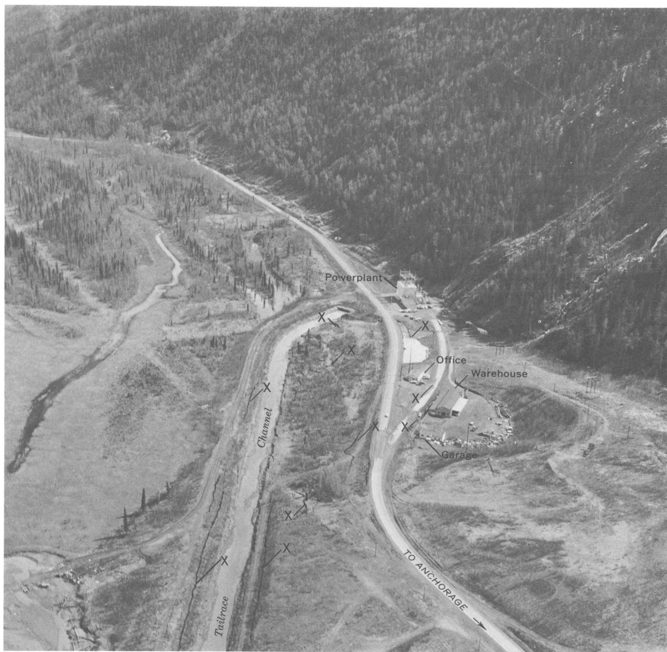
28.—Location of ground cracks in the vicinity of the powerplant.
