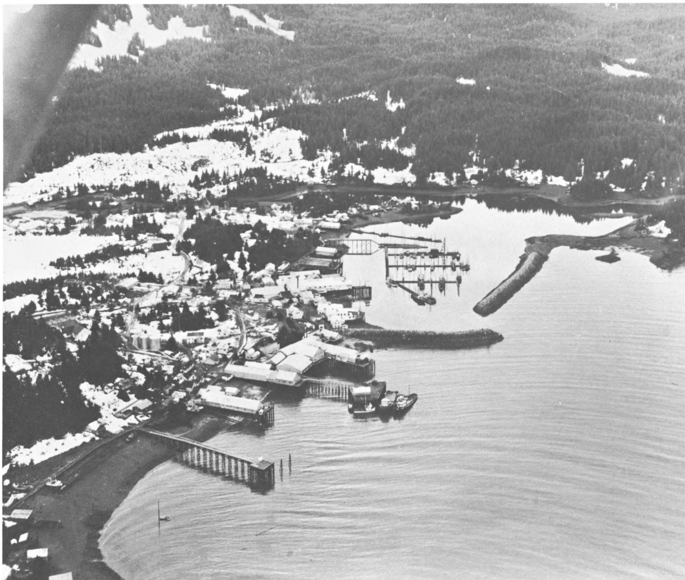
9.—Seldovia at low tide in March 1965, with raised breakwater and small-boat basin in use. Tectonic subsidence submerged boardwalk (curving structure at shore end of docks in foreground) at high tide. The boardwalk has been replaced on new fill. Urban renewal project will alter buildings and utilities to conform with higher water levels. U.S. Army photograph.
