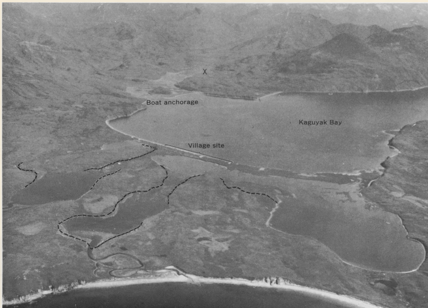
29.—Oblique aerial view of the head of Kaguyak Bay showing site of Kaguyak (fig. 28), approximate inland limits of debris deposited by seismic sea waves (dashed line), and location of small-boat anchorage. X marks position at which one 30-foot salmon trawler was stranded by the waves.
