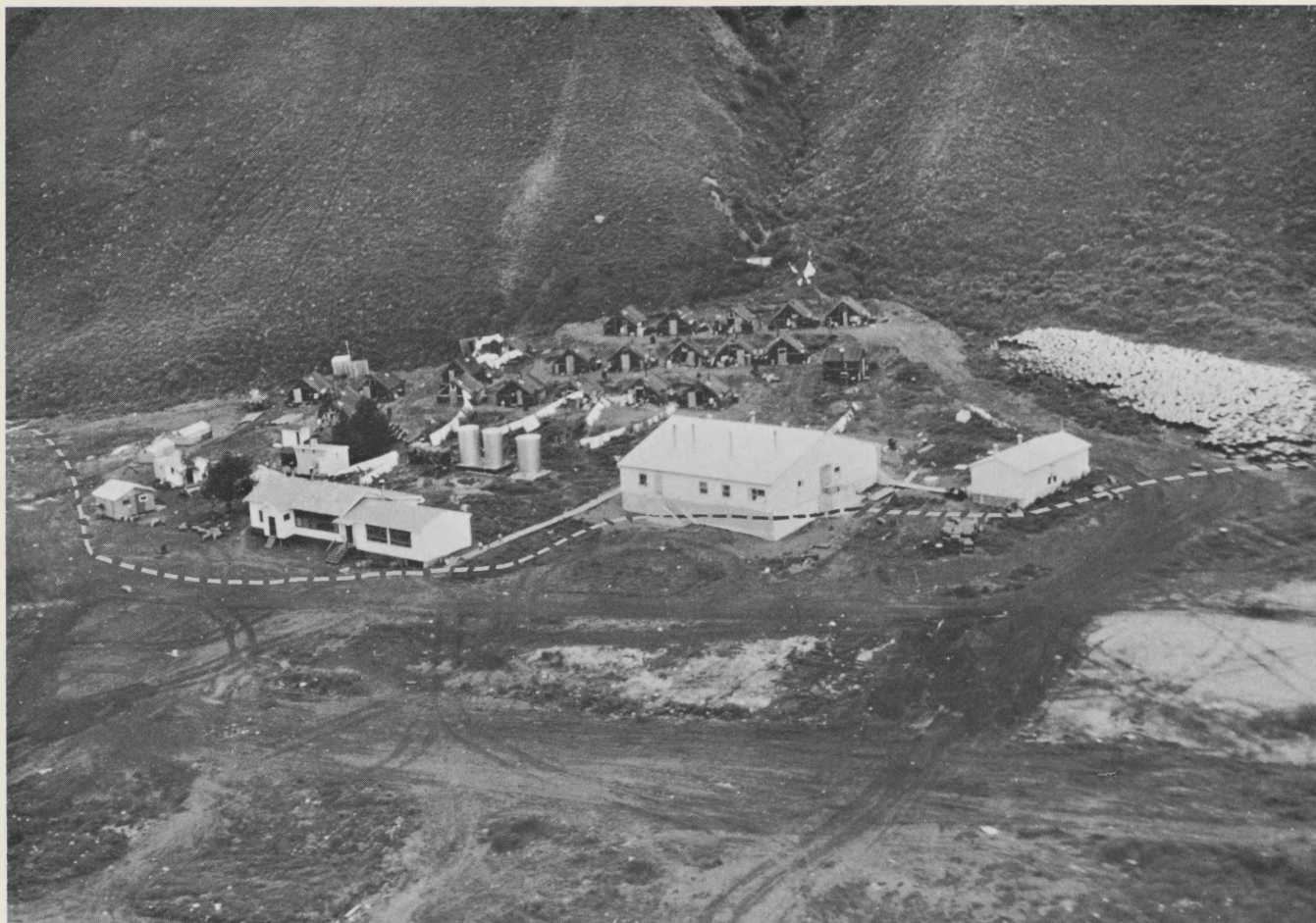
27.—Oblique aerial view of school area, Old Harbor, showing approximate inland limit of seismic sea wave inundation (dashed line). The area below the high-water line had been cleared of debris by the time this photo was taken (July 15, 1964). The structures near the apex of the alluvial fan are temporary shelters.
