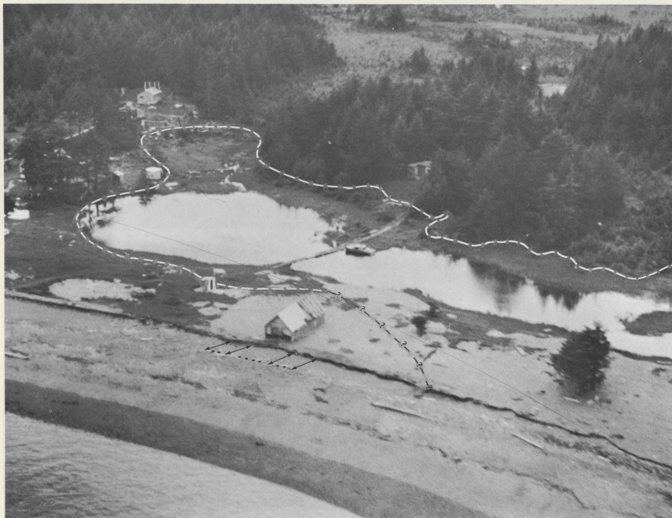
23.—Part of coast at Afognak. Arrows show approximate amount of landward retreat; newly formed beach berm is gray, and approximate extent of seismic sea wave inundation is indicated by dotted line. Note partly submerged automobile in pond.
