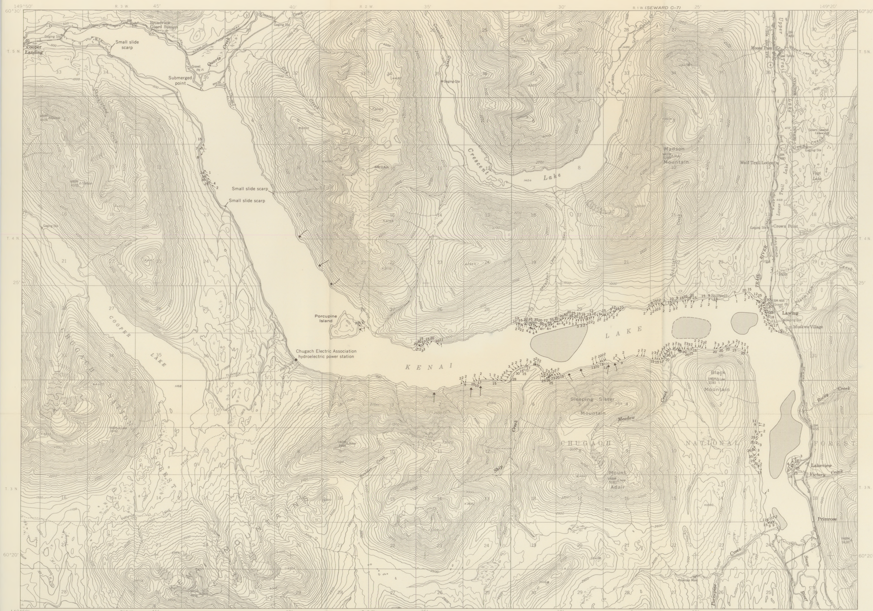
MAP OF KENAI LAKE, ALASKA, SHOWING THE DIRECTION, MAGNITUDE, AND RUNUP HEIGHTS OF WAVES, AND THE CHANGES IN THE SHORELINE THAT RESULTED FROM SLIDING DURING THE MARCH 27 EARTHQUAKE
