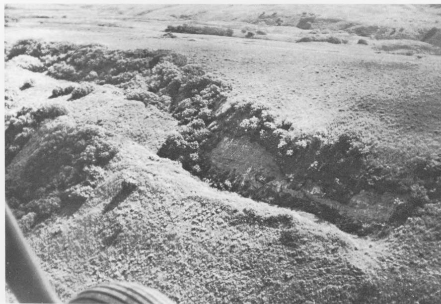
15. — Main scarp at the head of a large rotational slump in Tertiary deposits on Narrow Cape, Kodiak Island. The landslide is approximately 1,400 feet long and 125–150 feet high. The rock mass at the left slid 8–15 feet downslope along a surface of rupture, the main scarp of which trends diagonally across the photograph. Note the headward tilt of the original surface on the upper part of the slide mass and draping of the vegetation mat over the crown of the main slide.
