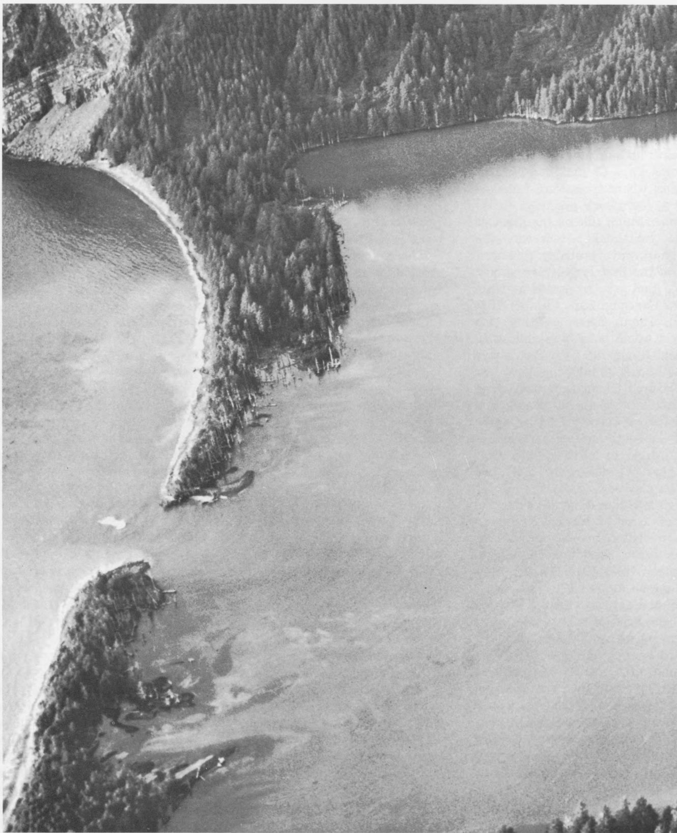
20.— Opening torn by seismic sea waves in the barrier beach of a large lake along the shore of Izhut Bay on Afognak Island. Channel scour and subsidence of at least 6 feet permit sea water to enter the basin at all stages of tide. Note partially submerged trees along inner margins of the beach spits, and small new rockslide along bluff in background. Photograph by Alaska Department of Fish and Game.
