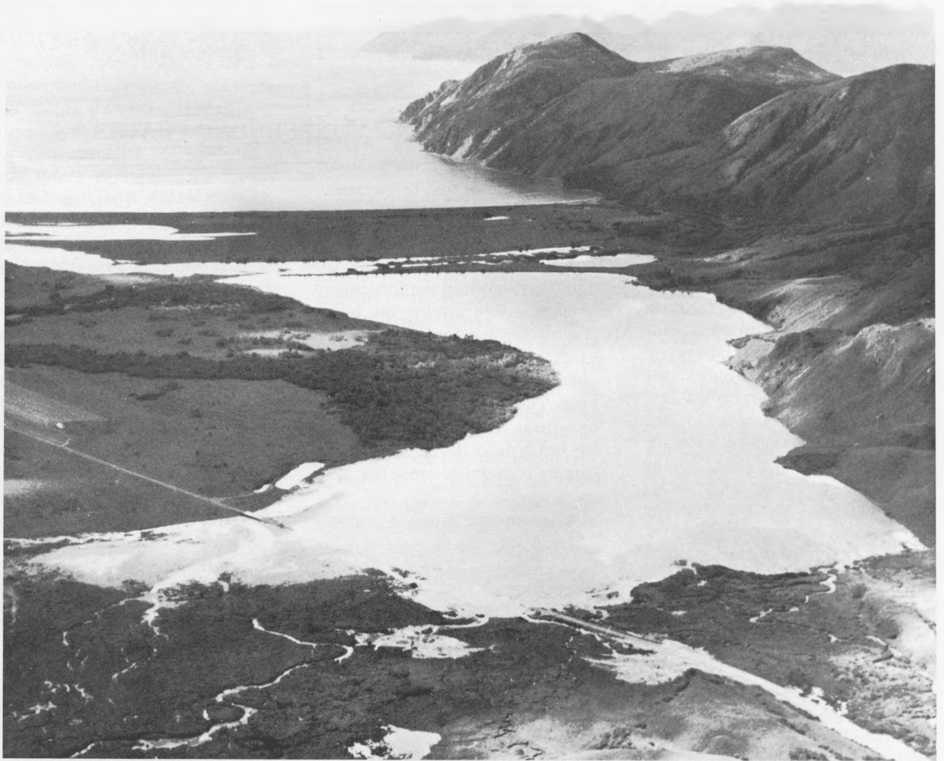
8. — Road near the head of Lake Rose Tead submerged by about 5 feet of surficial subsidence of inlet-stream deltaic deposits. Ugak Bay is visible in the background. Photograph by Alaska Department of Fish and Game.
