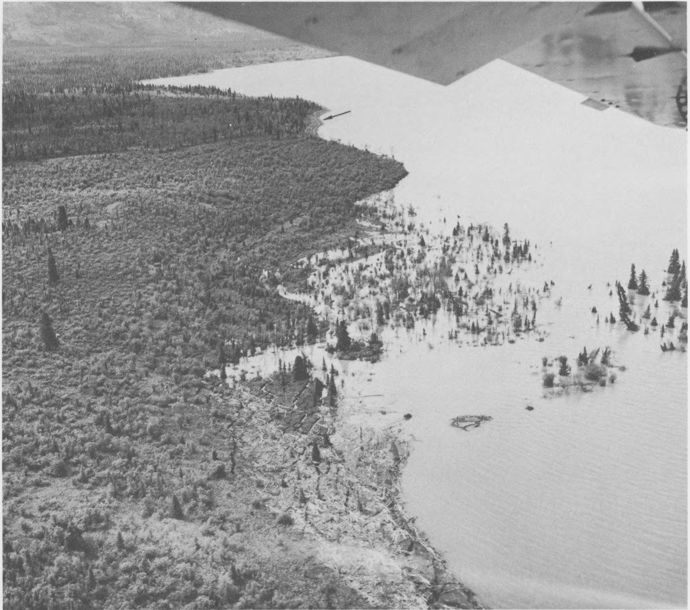
19.—Large inundated area along eastern shore of Tazlina Lake just south of the Kiana Creek delta. Lateral movement and vertical compaction of materials along lakeshore caused numerous ground cracks to form and the area to subside. Note normal beach (indicated by arrow) in the distance.
