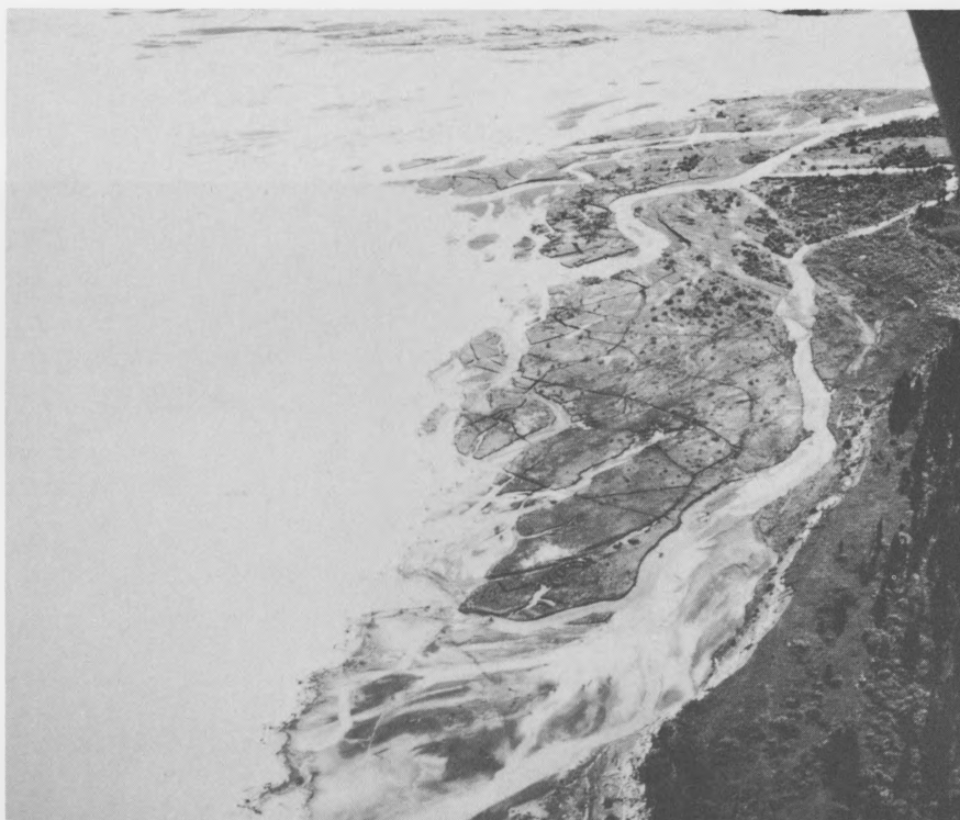
17.—North end of the large Nelchina River delta along the western shore of Tazlina Lake. Note the reticulate pattern of ground cracks which are as much as 6 feet wide.
