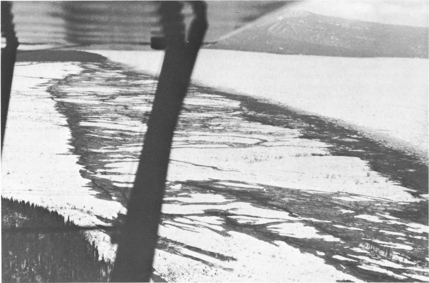
16.—Outwash delta at head of Tustumena Lake a few days after the earthquake. View is south (pl. 3). The ground was snow covered, and water and sand erupted along major cracks (dark-gray areas) partly removing the snow and covering the ground surface with sand. The cracked ice-covered lake surface is to the right. A major fissure system paralleling the delta front is seen to the left of center. Photograph by Avery Thayer, Fish and Wildlife Service, Kenai, Alaska.
