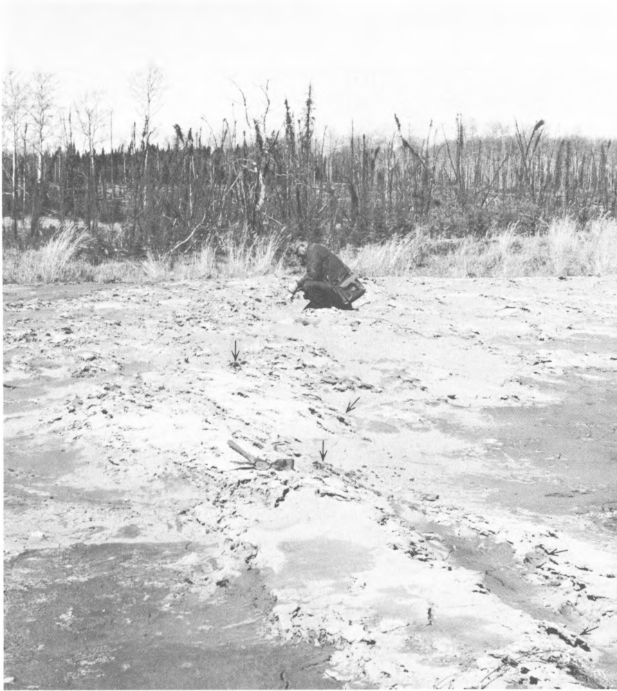
13.—Detrital coal extruded with sand (loc. 1, pl. 1). Copious amounts of sand were extruded from a fissure cutting a gravel road (loc. B. fig. 3). Pieces of coal and lignite as long as 6 inches (some indicated by arrows) were extruded with the sand.
