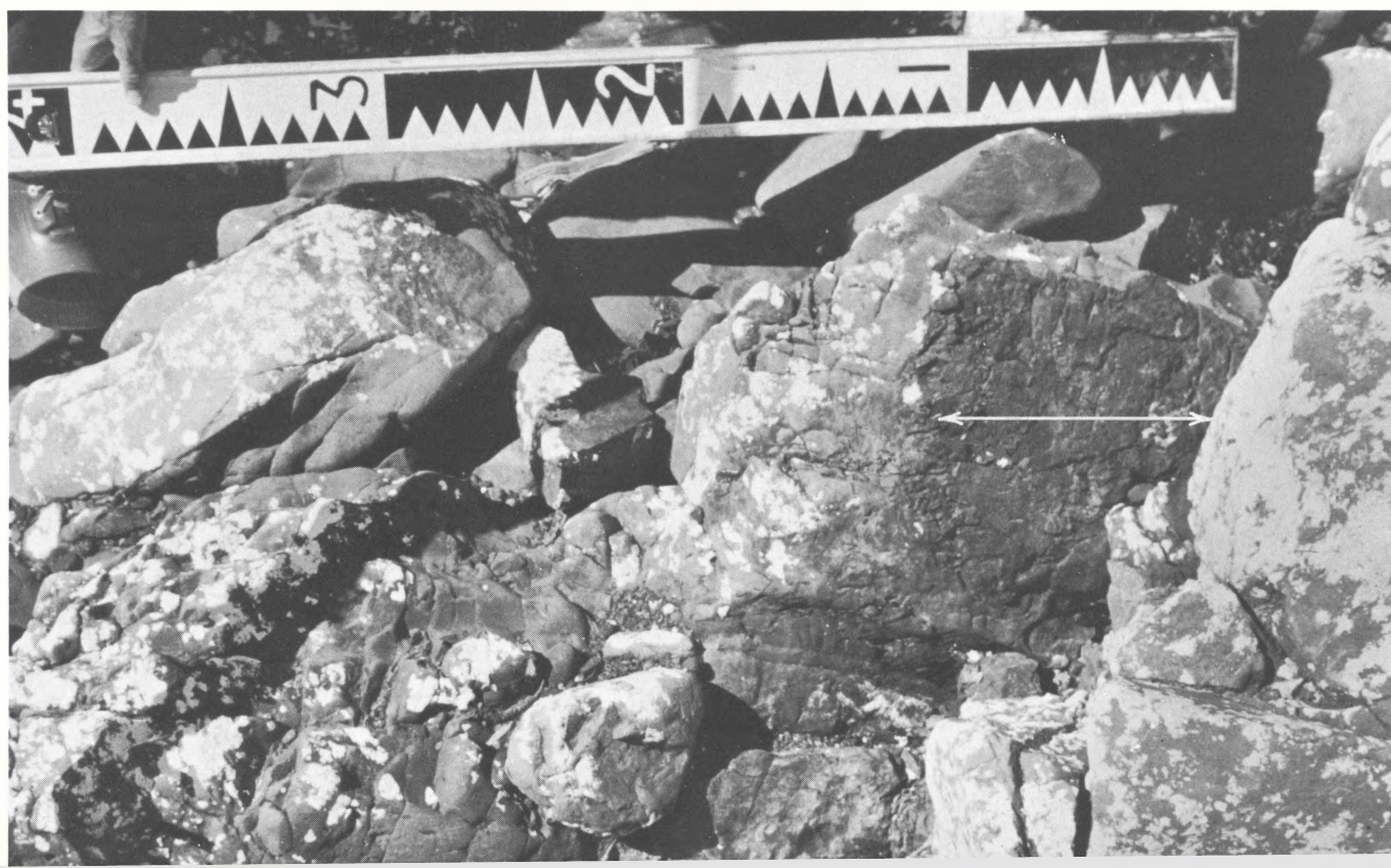
9.—Crack along bedding plane in massive indurated sandstone; 1 foot of left-lateral separation. Location shown in figure 6.
