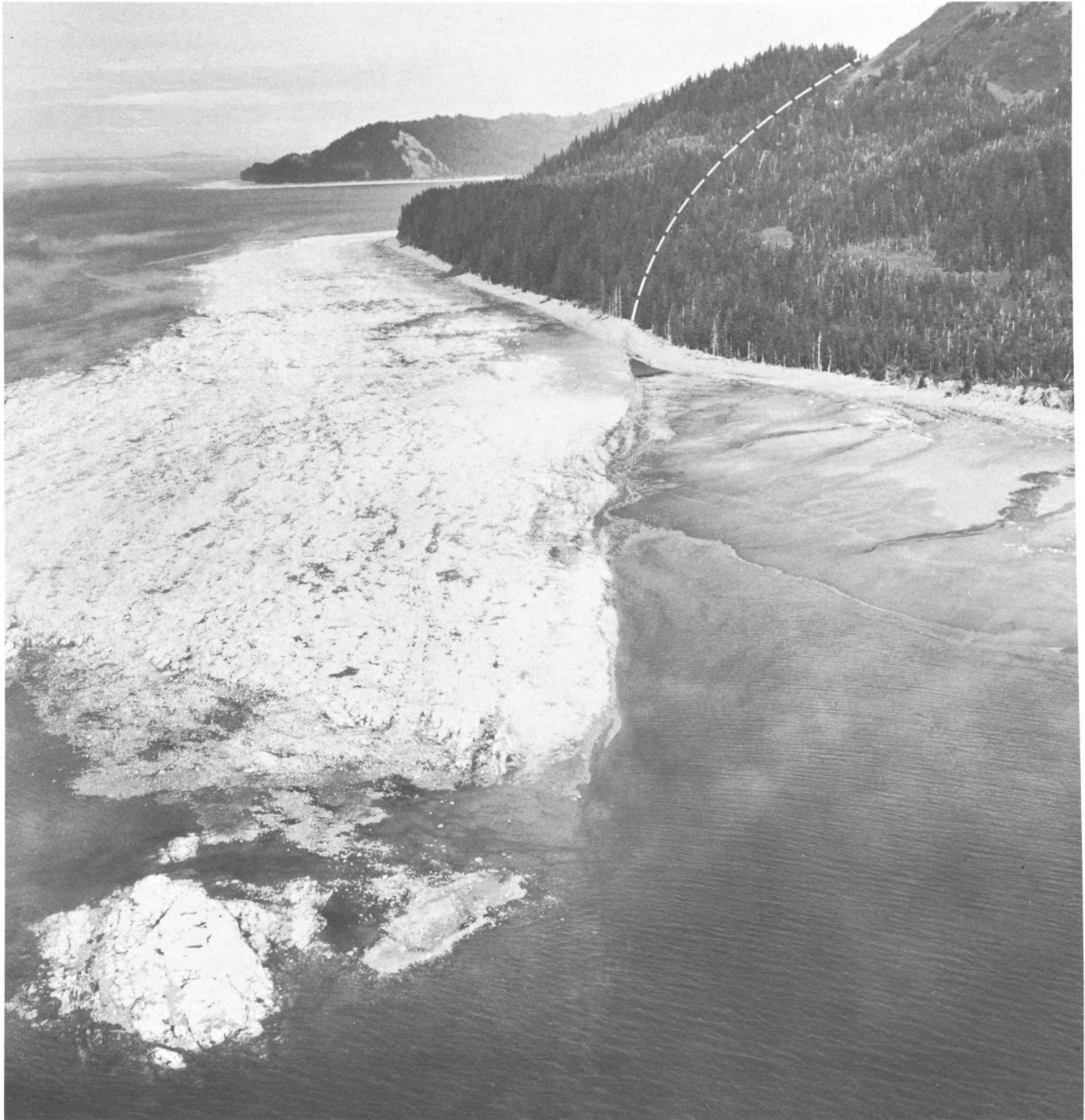
35.—Hanning Bay fault north of Fault Cove. The average 65^{\circ} -NW. (left) dip of this segment of the fault causes the trace (dashed) to be deflected uphill (right) as it crosses the 850-foot-high ridge between Fault Cove and Hanning Bay. The pond, at the intersection of the fault scarp and the former beach ridge, occupies a closed tectonic depression in the downthrown block.
