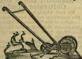
The "Planet Jr." Combined Drill, Cultivator and Plow.
