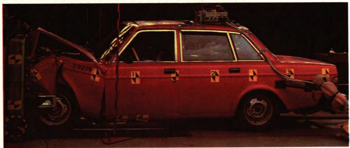
"A barrier impact at 35 mph can generate between 80,000 and 120,000 lbs of force."
