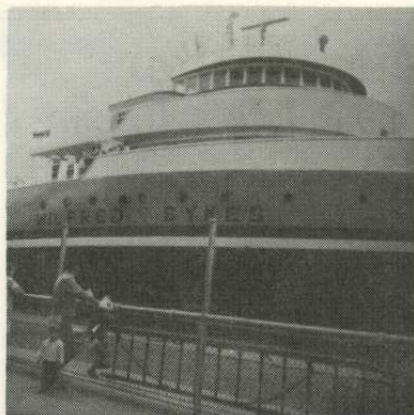
The Wilfred Sykes, a huge bulk carrier owned by the Inland Steel Co., comes through one of the Soo Locks at Sault Ste. Marie. This is just the front end — the overall length is 678 ft. It is 70 ft. wide and has a capacity of 21,800 tons.
