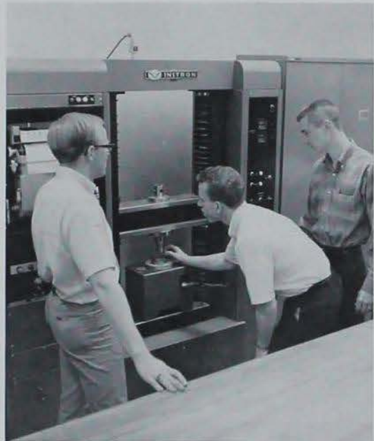
In this ceramics lab, students are working with an Instron, a device for making tensile tests.
