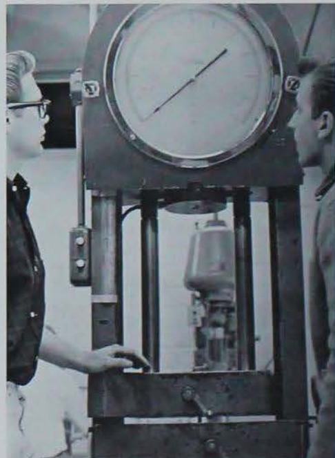
Mechanics students check the tensile strength with a machine that applies a measured force to metal bars.
