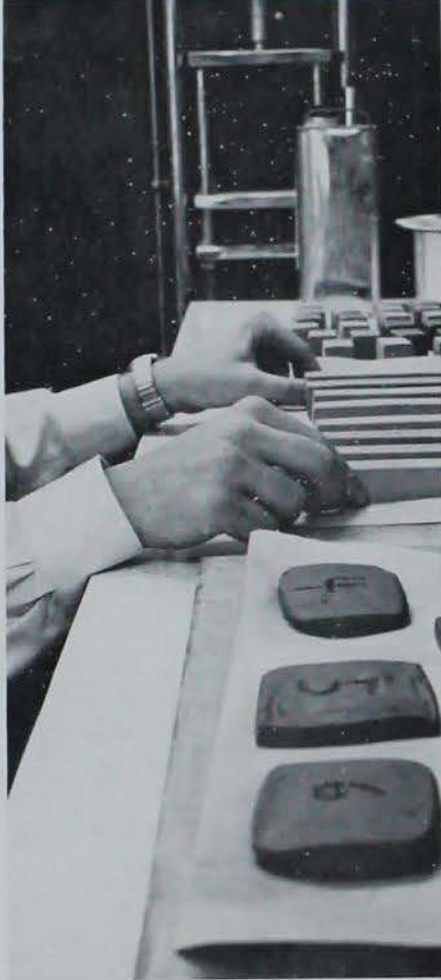
A ceramic engineering completes the last of many checks on brick samples before firing in the kiln.
