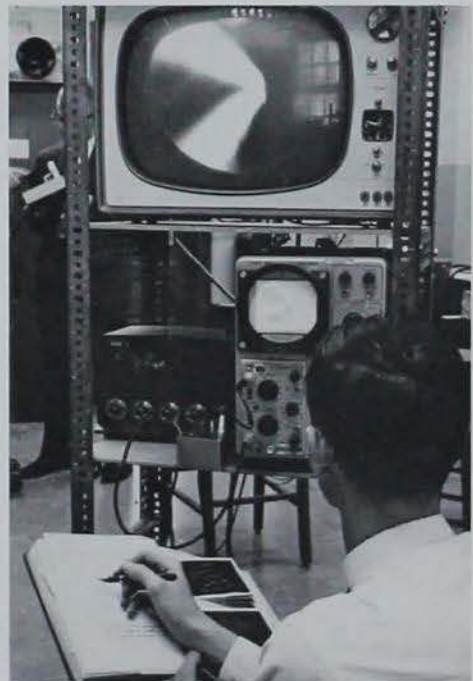
Engineers doing photoelastic studies of microscopic stresses in sodium chloride crystals use TV monitors.
