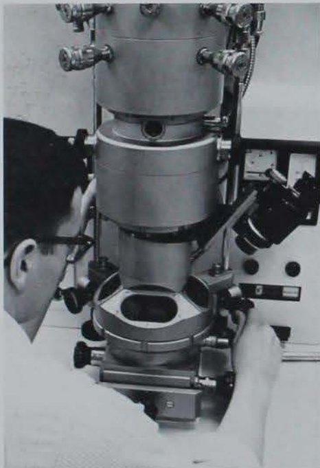
The Siemens electron microscope, used for engineering research, is capable of 160,000x magnification.
