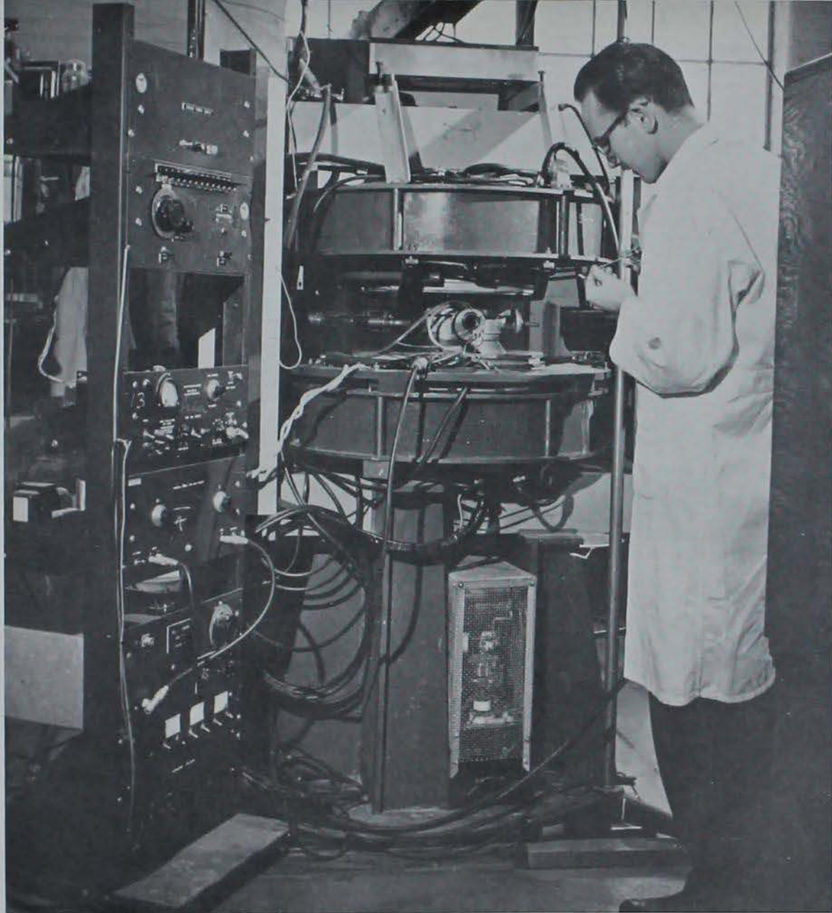
PHYSICS GRADUATE STUDENTS work with the Iowa State Cyclotron which accelerates protons by use of magnetic and electrical fields to cause a nuclear reaction.
