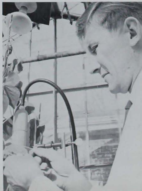
WORKING for a Ph.D., Douglas Laing measures the internal water status of leaves by recording beta count omissions from injected C-14.
