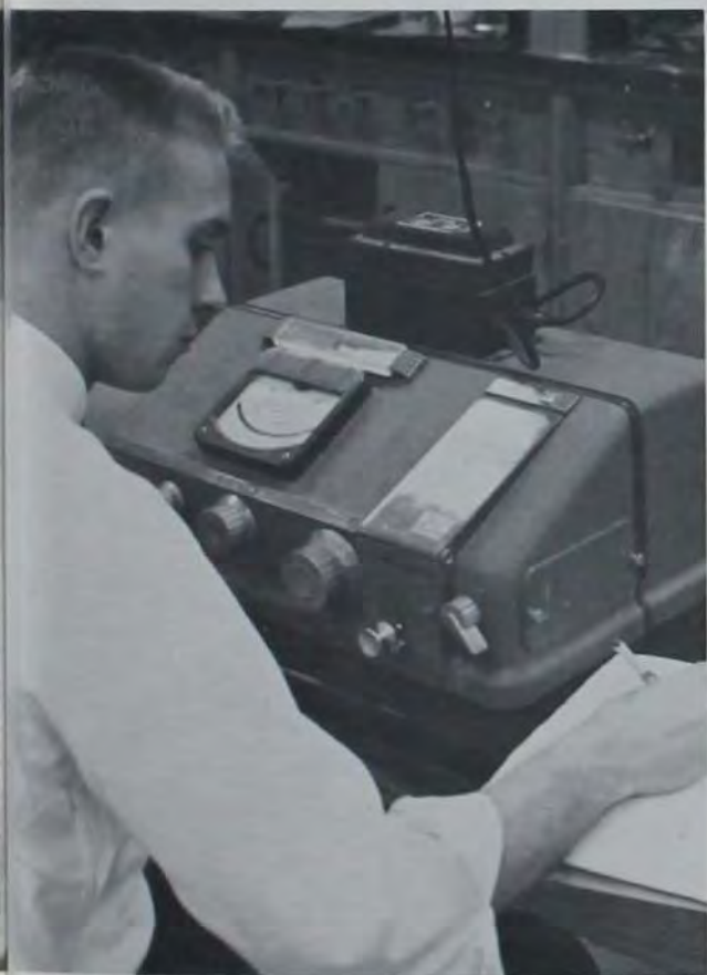
MEASUREMENT of the absorption spectrum of hemoglobin is done by a student in biochemistry using a spectrophotometer.
