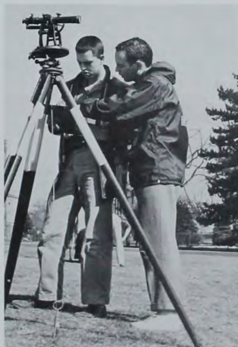
DON LINN and Luis Gonzales record measurements made with the transit in a surveying class offered to landscape architecture and forestry students, as well as those students of the civil engineering department.
