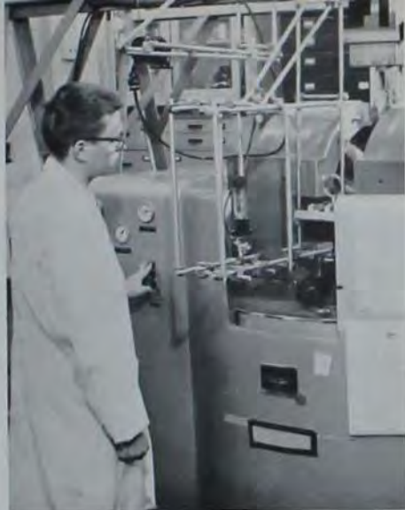
LEWIS BARTEL, graduate assistant in physics, is determining absorption spectra of single crystal of rare earth ethyl sulfates by means of a Littrow-Echelle spectrograph.
