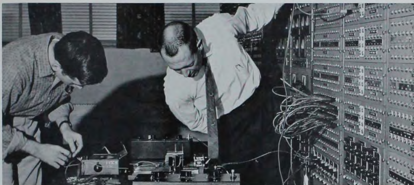
KENNETH KRUEMPEL, electrical engineering graduate student, and Dr. Paul M. Anderson attempt to coordinate the network analyzer with a Hall Effect wattmeter, a research project built from components by Kruempel.
