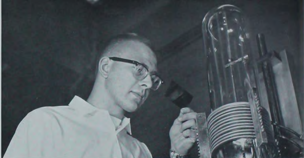
PASSAGE of a molten zone along a bar of vanadium metal in a high-frequency furnace enables metallurgy graduate assistant, Robert Thompson, to prepare high-purity vanadium.
