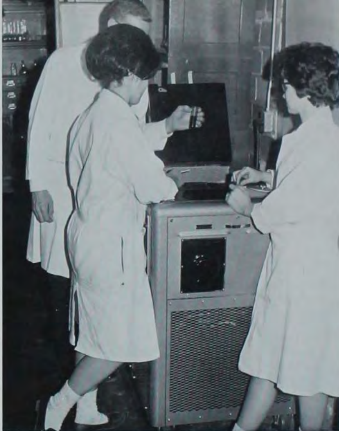
ANALYTICAL WORK in the poultry laboratory is aided by the use of the new refrigerated centrifuge.
