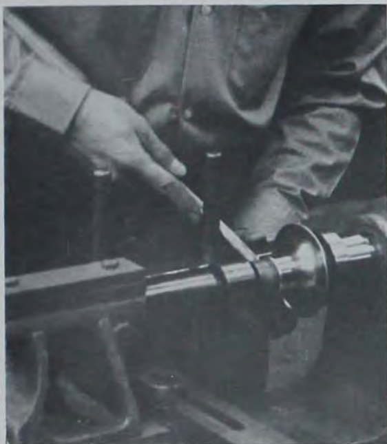
PROFICIENCY IN SHOP WORK, such as this using of a metal spinning lathe, is necessary for I.Ed. majors who will be transmitting this proficiency to students in both school and industry.
