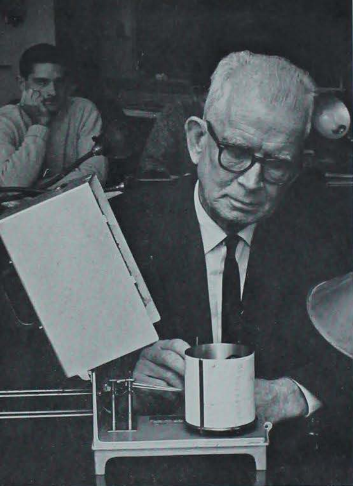
IN A PLANT ecology lab, Dr. John Aikman demonstrates a thermograph, a device for automatic temperature recording.
