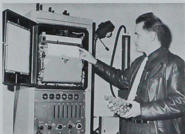
X-RAY DIFFRACTION machines are used by soil researchist, Dr. Handy, to identify minerals and to study crystal structures.
