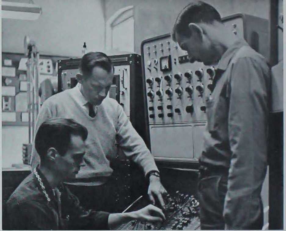
TO SIMULATE a stability change of a missile is the goal of these aerospace engineering students who are setting up an analog computation program.
