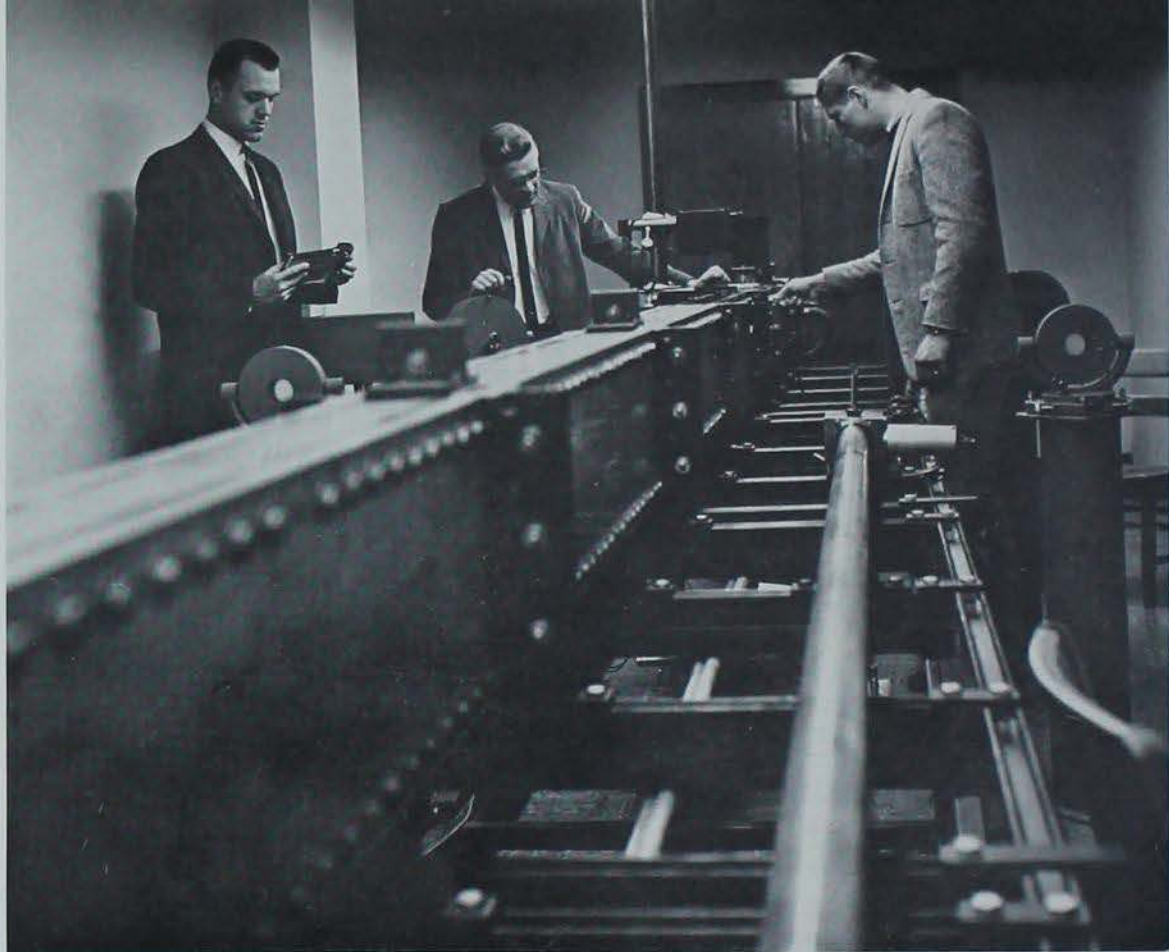
NATIONAL SCIENCE Foundation undergraduate research participants Jan Spelman, Wayne Franzen, and John Felderman shoot gas at sonic velocity to study thermodynamic propulsion of gases before and after shock waves.
