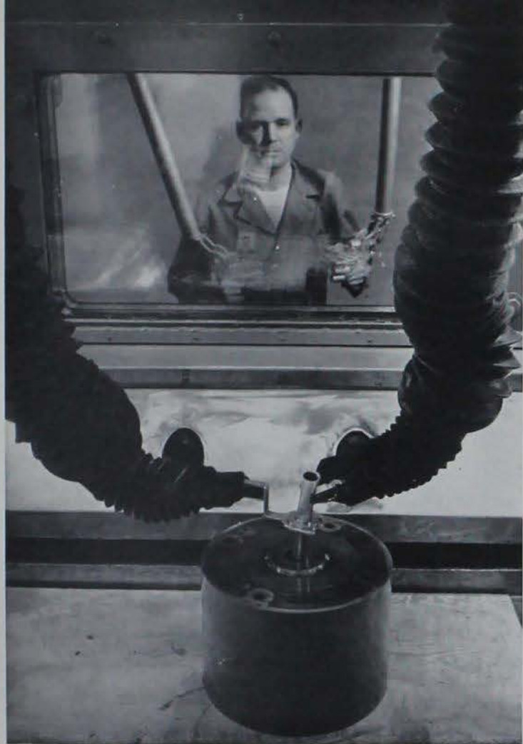
Remote control "hands" are a must when handling highly radioactive material involved in atomic research in the Ames Laboratory sponsored by the Atomic Energy Commission.
