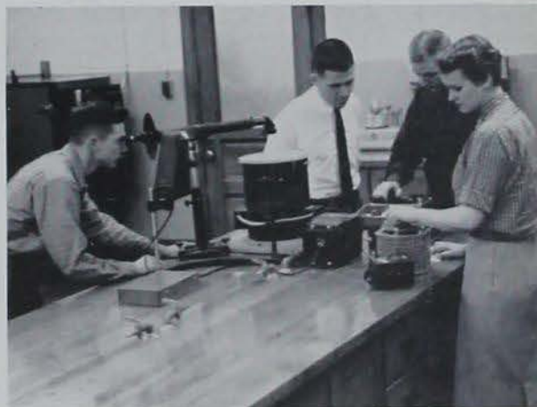
Students in one of the division's smaller departments, ceramic engineering, check by means of a spectroscope the coefficient of expansion of substances at high temperatures.
