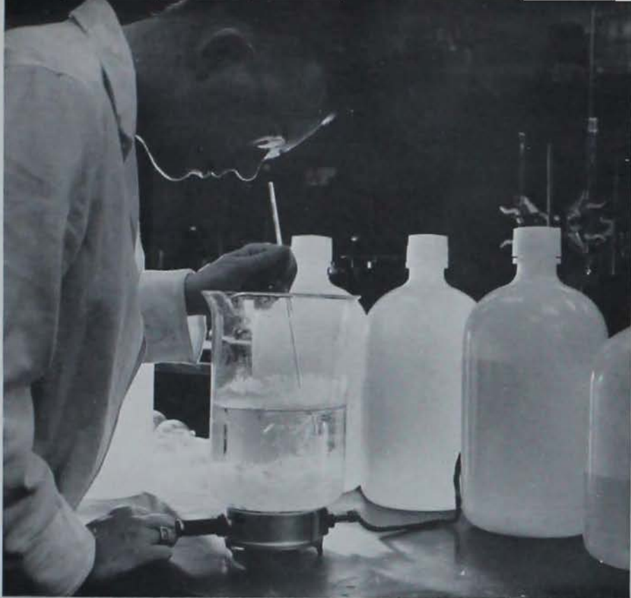
LEONARD DRUDING, chemistry graduate student and assistant at the Ames Laboratory, crystallizes potassium nitrate for use in kinetic studies.
