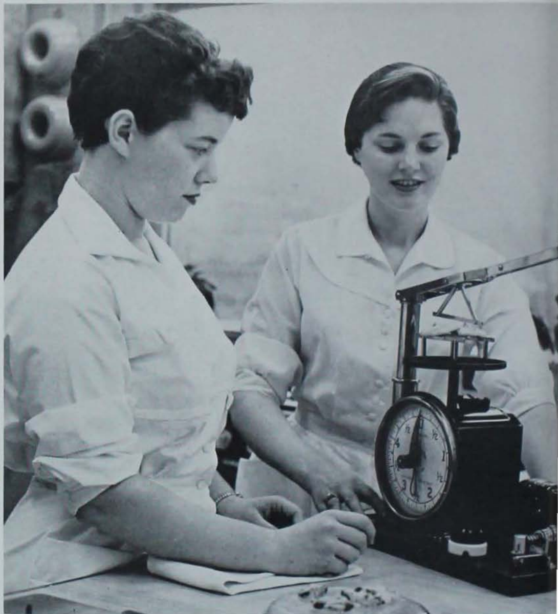
GEORGIA GASKILL, left, and Marysue Kritzman, seniors in experimental foods, use a shortometer to test the strength of a cookie. The measure is one of several tests used on products developed by students in experimental foods.
