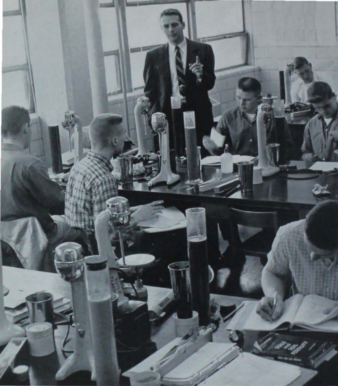
BY USE of the George Bouyoucos analysis procedure, students in a freshman agronomy class are able to determine the percentage of sand, silt and clay in a variety of soil samples.
