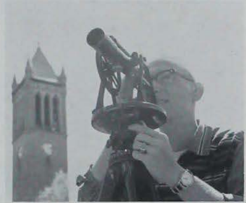
ENGINEERING STUDENTS work outside as well as inside. Here Alden Lude uses his transit to give a line up to the chainman.
