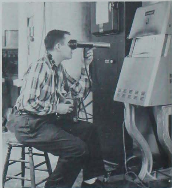
MICK MARLOWE, ceramic engineering major, operates an optical pyrometer, which measures the temperature of the furnace.
