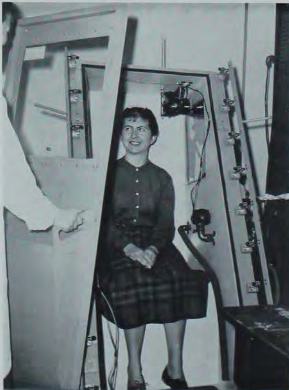
MARGARET McKINNEY, home economics graduate student, takes her place in a helium chamber, an experimental apparatus used to measure body volume.
