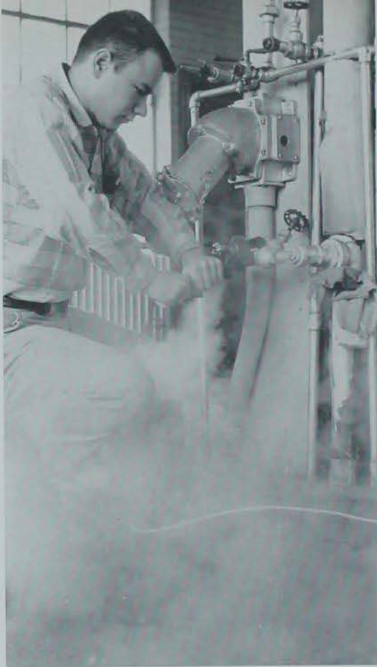
RUNNING A STEAM quality test is Jim Grey, a senior majoring in chemical engineering.
