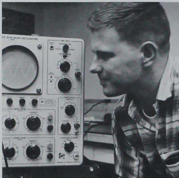
ELECTRICAL ENGINEERING student Richard Gowen uses an oscilloscope to observe the deflection of a beam of cathode rays.
