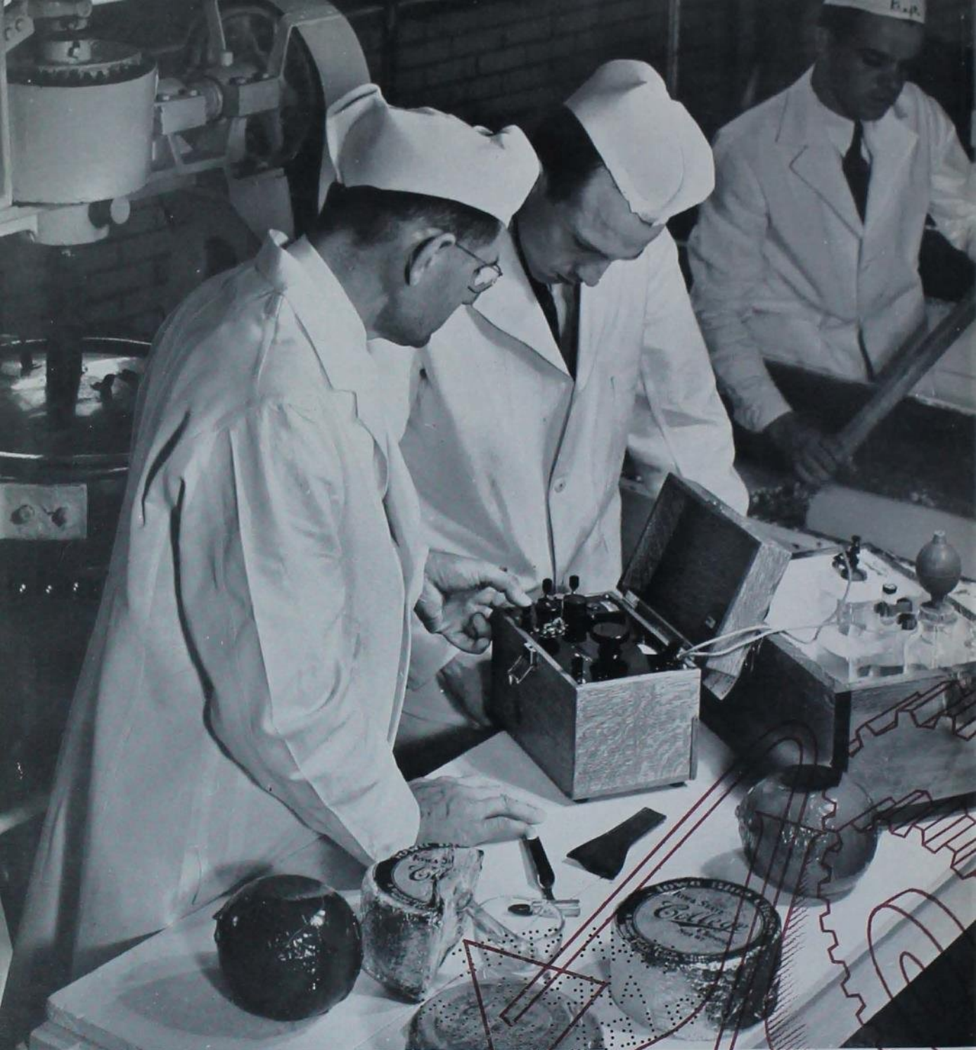
In obtaining the highest quality of cheese the determination of hydrogen ion concentration electrically is made by the potentiometer.
