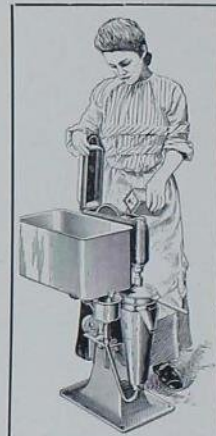
OILING THE DAIRY TUBULAR
